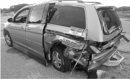
Figure 2 Post-crash at 50mph failed
